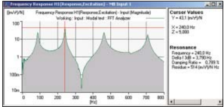
Fig. 2 Magnitude of one of the accelerance functions. Resonance frequency and damping is extracted for the 2nd mode
